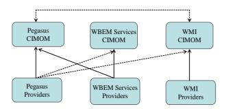
Figure 10. The Compatibility between WBEM Implementations
