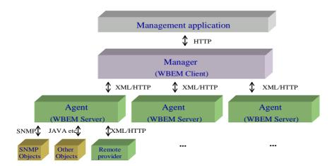
Figure 4. Overall Management System Architecture
