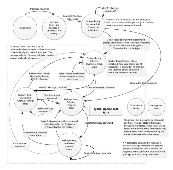
Figure 6 - NC-SI operational state diagram
