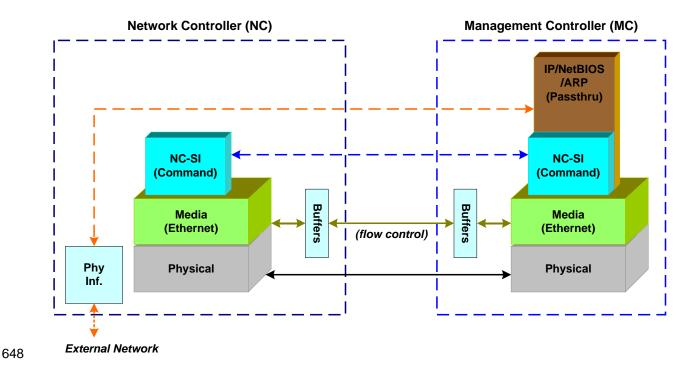
Figure 5 - NC-SI transport stack
