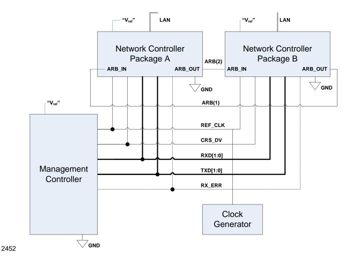
Figure 16 – Example NC-SI signal interconnect topology
