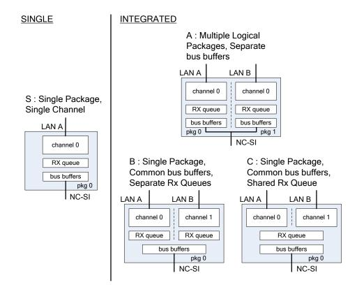
Figure 4 - Network Controller integration options
