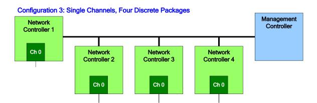
Figure 3 – Example topologies supported by the NC-SI
