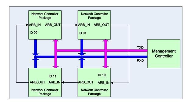
Figure 11 – Multiple Network Controllers in a ring format
