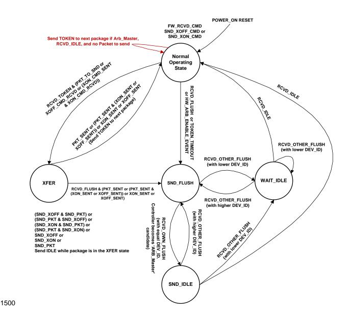
Figure 14 - Hardware arbitration state machine
