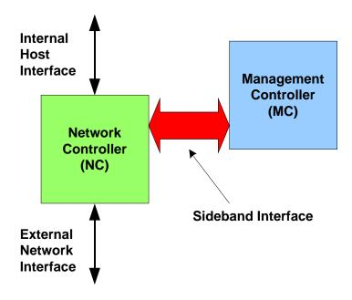
Figure 1 - NC-SI functional block diagram
