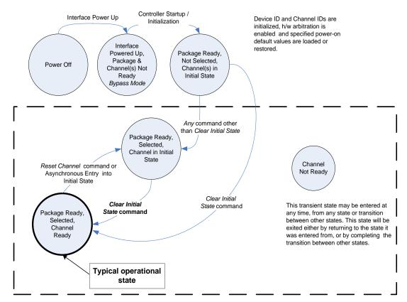
Channels within the controller (package) can independently enter and exit their respective Channel States.
