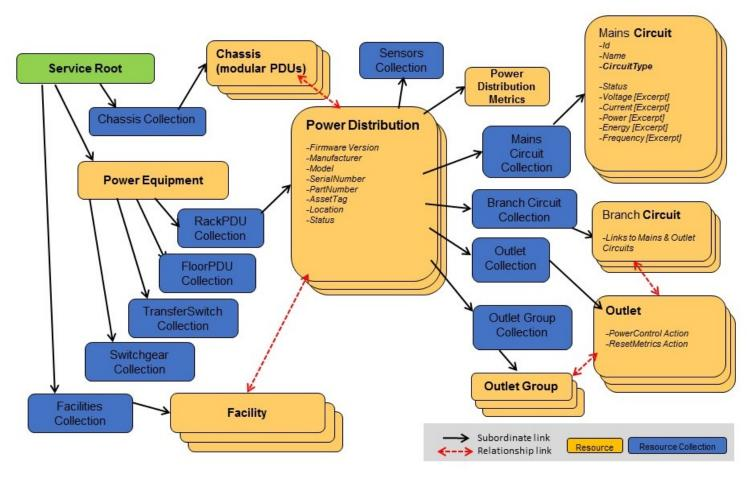
Figure 1: Resource Tree for a Power Distribution Unit
